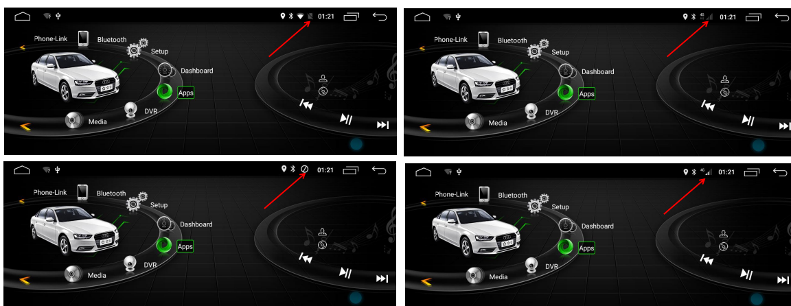
Figure 1: ① no SIM card is inserted, 4G antenna is not connected.
